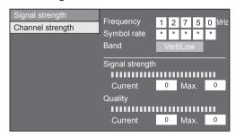
Position and align the antenna so that the maximum possible values for "Signal strength" and "Quality" are obtained.
